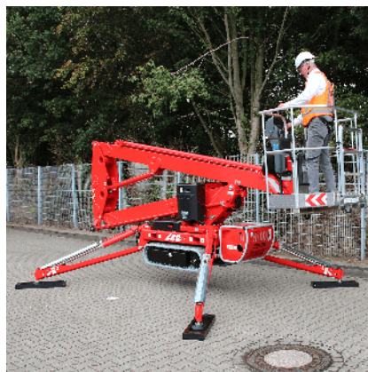
Automatic self-levelling stabiliser system
